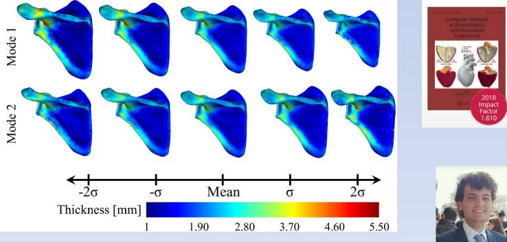
Shape and cortical thickness variation in the first two modes of variations. For mode 1 (top), when passing from a large scapula ( $-2\sigma$ ) to a small scapula ( $+2\sigma$ ), a decrease in cortical thickness is visible. Mode 2 (bottom) shows a variation in the glenoid inclination and acromion orientation, with no visible relation to the cortical values."
